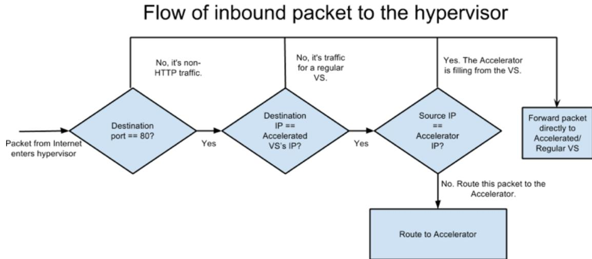
OnApp Accelerator has a built-in monitoring and failover mechanism. Should the Accelerator VS appliance malfunction, the *ebtables* and *iptables* rules are removed, and HTTP/HTTPS requests are immediately routed back to the target VM.
